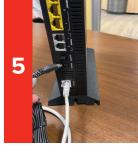
Plug the power cord into the black port that says, "POWER" on the back of your router then plug it into a regular outlet.
